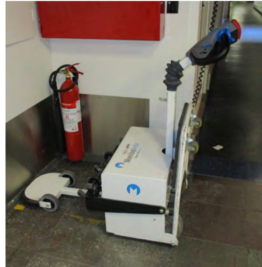
Figure 4: MoovingBeds , a supporting tool for the transportation of beds at Odense University Hospital.
