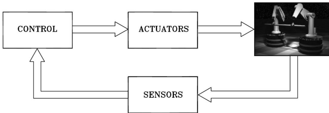
*Figure 1 Components of a robotic system [2]*
