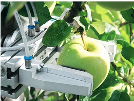
Festo developed the cutting and gripping devices for the CROPS project: “The aim is a configurable, modular and intelligent robot platform, which reliably recognises both the fruit as well as obstacles and other objects.”
