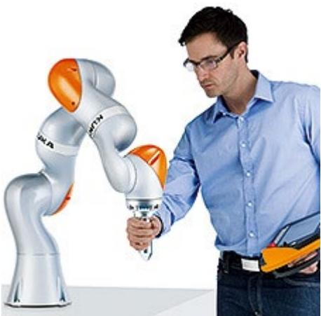
KUKA has developed industrial arm robots, including the LBR iiwa, which stands for "lightweight robot, intelligent industrial work assistant". This light payload industrial arm offers the “highest form of human-robot collaboration in industry” and includes collision detection.
